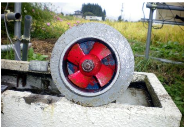
Pic2. turbine of hydroelectric system
